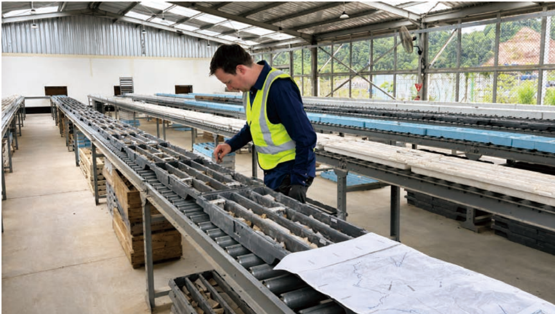
Figure 6-6 Core Inspection by Competent Person during Pani Site Visit
